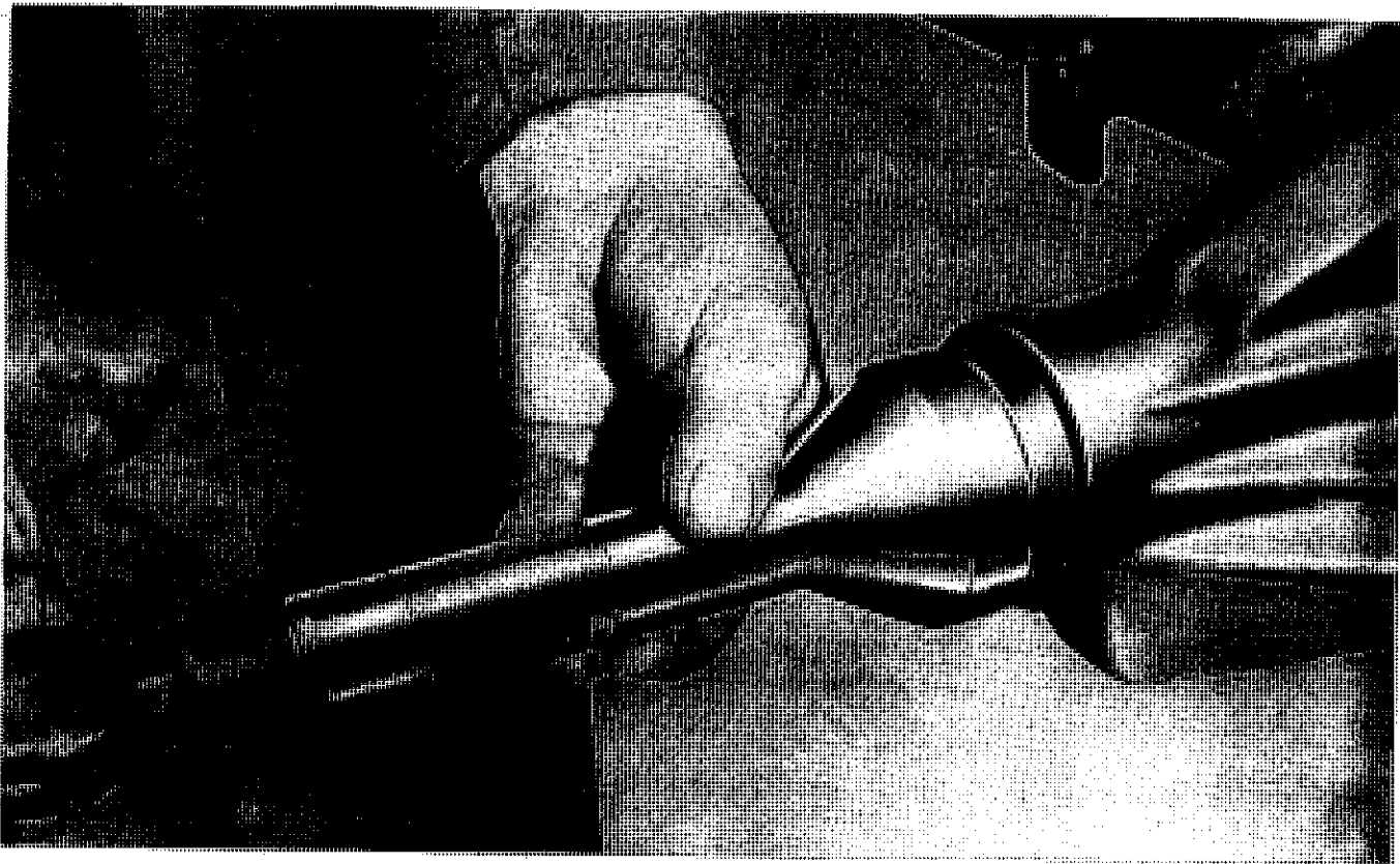
Fig. 23. Fitting Pinion Oil Seal—Tool No. M.100.
