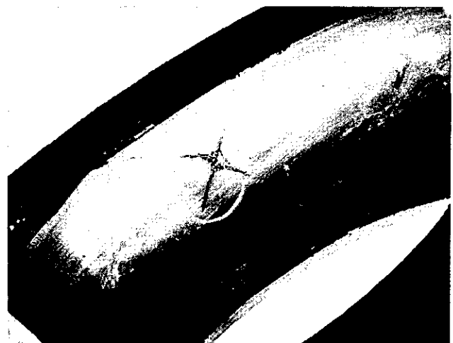
Fig. 8. Impact fracture caused by striking a sharp object such as a brick-end or pavement kerb
